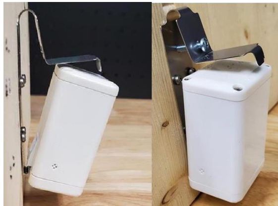
Figure 2-3: Attaching the Tracker to the Mounting Bracket
