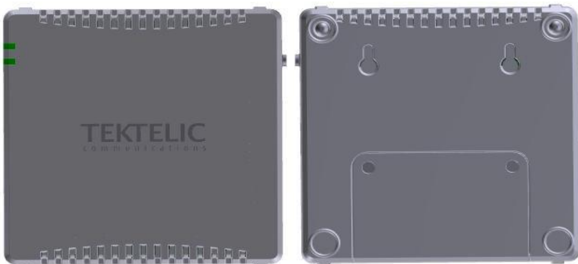
Figure 4: KONA Micro Gateway Module Wall Mounting Orientation
