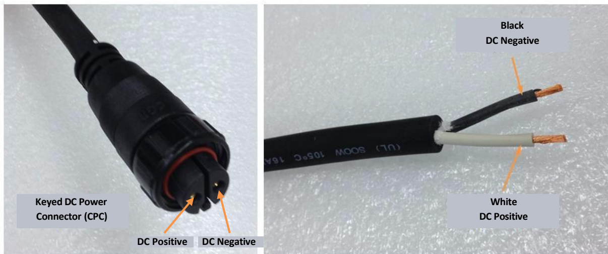
Figure 6: Direct DC Power CPC Connector Connection Polarity
