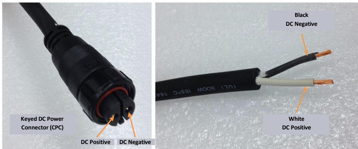
Figure 6: Direct DC Power CPC Connector Connection Polarity
