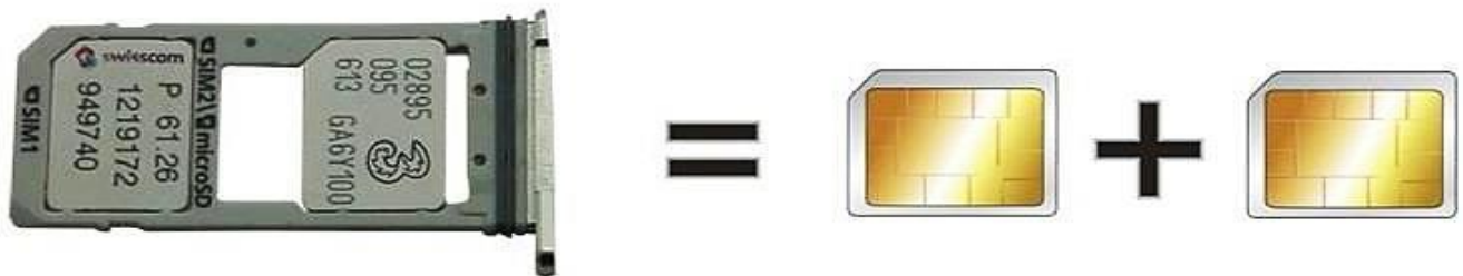
Figure 4: SIM Tray Layout
