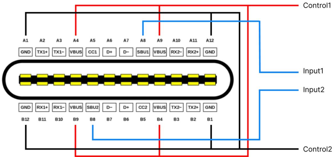
Figure 1-1: USB-C External Connector Pin Layout
