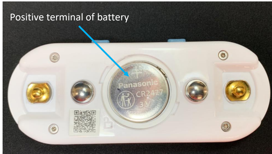
Figure 3-3: Placing battery in device
