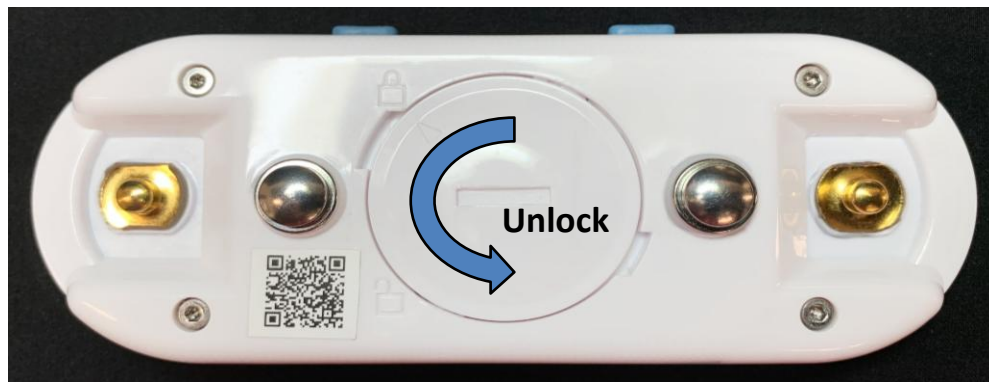
Figure 3-1: Unlocking battery lid
