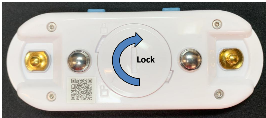
Figure 3-3: Placing battery in device
