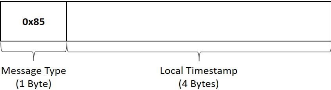
Figure Appendix 0-13: Frame format of local timestamp acquisition request in an UL payload.
