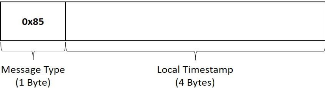
Figure Timestamp Acquisition Stream-8: Frame format of sensor timestamp response in an UL payload.
