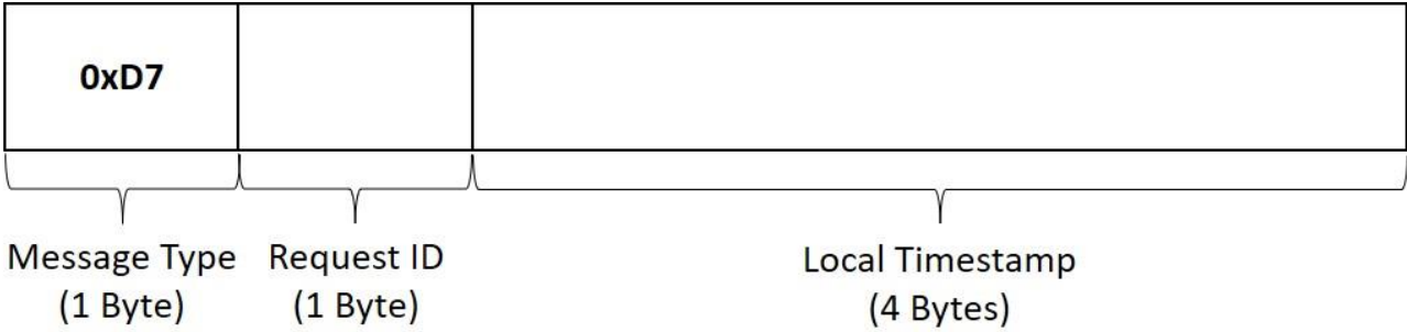
Figure Appendix 0-16: Frame format of local timestamp acquisition response in a DL payload.
