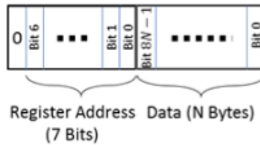
Figure General Sensor and LoRaWAN Communication Information-5: Bit Indexing Scheme for Configuration Registers
