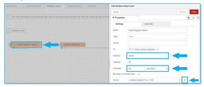
6. Deploy changes. After that you can activate push button to read the Modbus register values.
