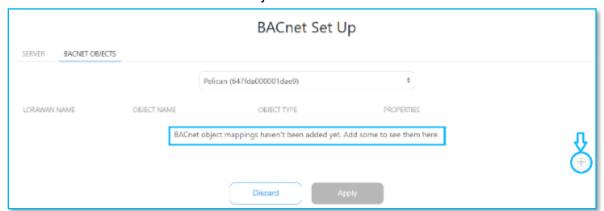
b. User can enter the LoRaWAN Name (ensuring it matches the parameter name used in the LoRaWAN decoder), along with the Object Name, Object Type, and Properties (such as units).
