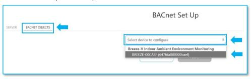
**NOTE:** BACnet objects are automatically be created upon receiving an LoRaWAN Uplink. Alternately, users may follow "Manual configuration of BACnet Objects" steps to setup BACnet objects.
