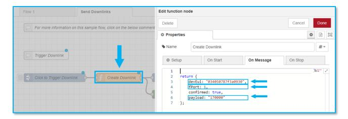
8. To get the DevEUI go to **Application** section in Embedded LNS and pick the application. In Devices section pick the **DevEUI** of the Device.
