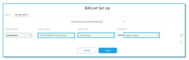
d. The Object Type for an Uplinks are typically Multi-state Input, Character string value, Analog Input, or Binary Input. Object types used for downlinks are typically Analog Value, Binary Value, Character String Value, or Octet String Value.
