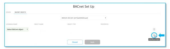
b. Select the BACnet object, i;e the LoRaWAN parameter name from the drop down.
